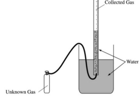
A sample of an unknown gas from a cylinder is collected over water in the apparatus shown above. After all the gas sample has been collected, the water levels inside and outside the gas collection tube are made the same. Measurements that must be made to calculate the molar mass of the gas include all of the following EXCEPT
